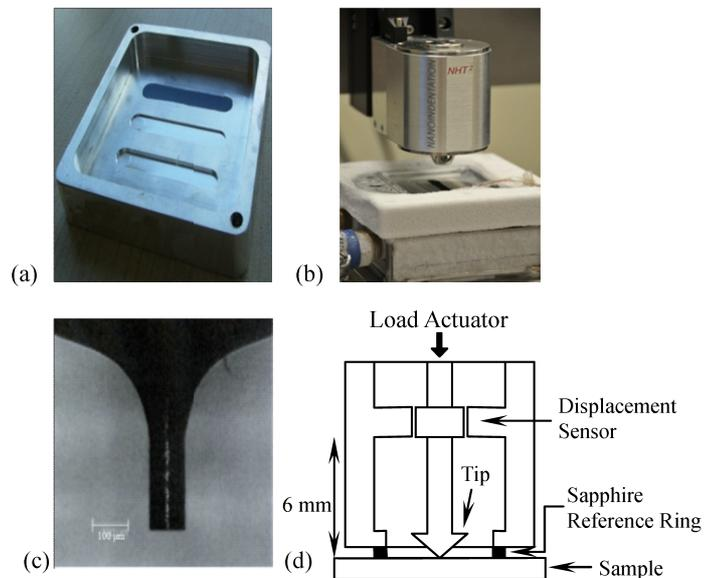
**Fig. 1.** (a) Sample tray with the 200 micron trough filled with asphalt; (b) Indenter module positioned above the frosted cold stage; (c) Optical image of the 100 micron flat-ended punch; and (d) Schematic of the internal configuration of the CSM NHT<sup>2</sup> indenter head.
