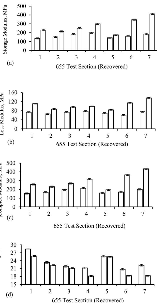
**Fig. 5.** Dynamic rheological data for recovered binders at 0.5 Hz and -8°C (first column) and -14°C (second column): (a) Storage moduli; (b) Loss moduli; (c) Complex moduli; and (d) Phase angles. Note: Error bars reflect ± 1 pooled standard deviation.
